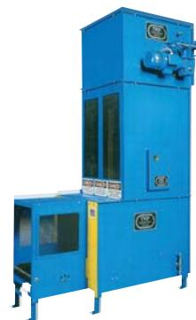
smooth-bottom unit loads up to 50 pounds. The conveyor platform consists of interlocking molded polymer flights with steel connecting pins. The conveyor lifts at a maximum
